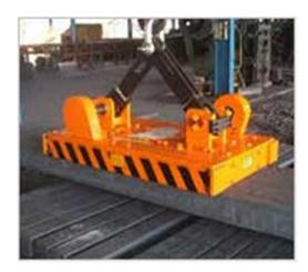
Our large lifting magnets are designed for applications such as handling billets, bundles, bar stock, slabs, plates, structural, long bar stock, rail, hot material, coils, pipe rebar, radioactive material, slag, and more.
